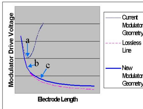
Figure 2. Modulator Driver Voltage versus Electrode Length
