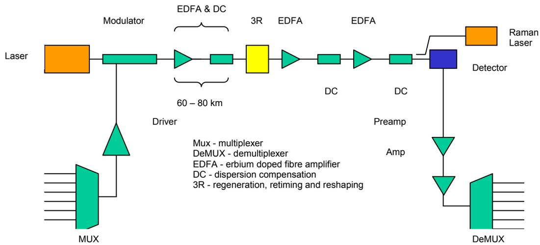
Figure 1. Simplified Schematic of a Long Haul Communications Network
