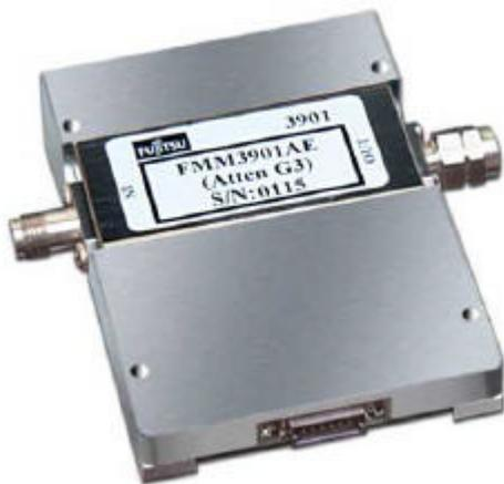
**Figure 1.** Photograph of the LN driver module. The RF section of the module contains the MMIC amplifiers and high frequency components. The bias and loop control circuitry are provided on a PC board within the housing.
