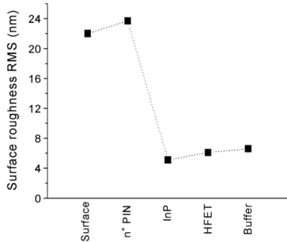
Fig. 2: Surface roughness of different layers after various etching processes
