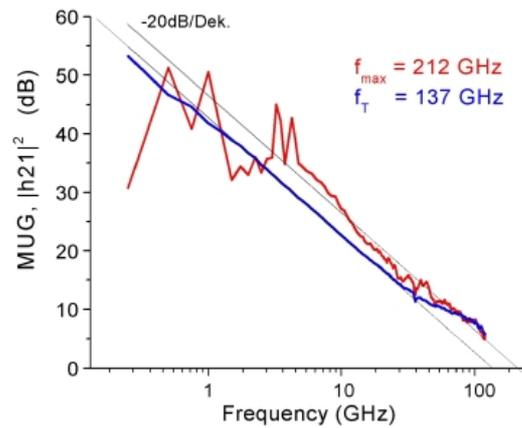
Fig. 4: Measured s-parameters of the 2x60 μm heterointegrated MHFET
