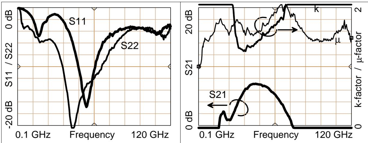
Fig. 5: Measured s-parameters of the single-stage amplifier
