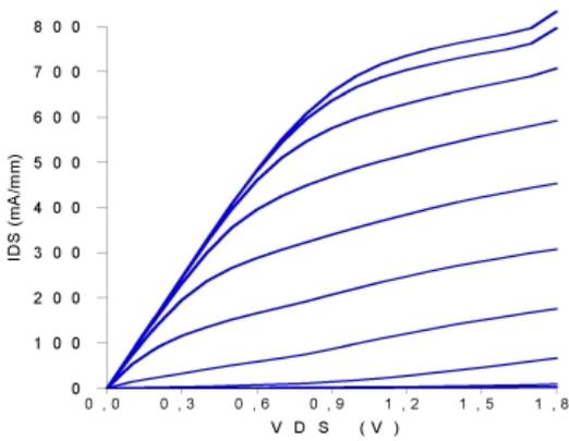
Fig. 3: Output characteristics of the 2x60 μm heterointegrated MHFET
