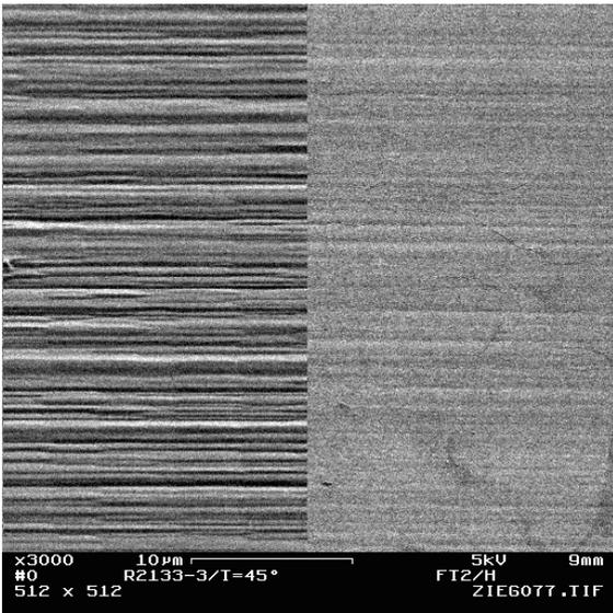
Fig. 1: SEM picture of surfaces on top of the layers (left) and on the etch stop layer (right)
