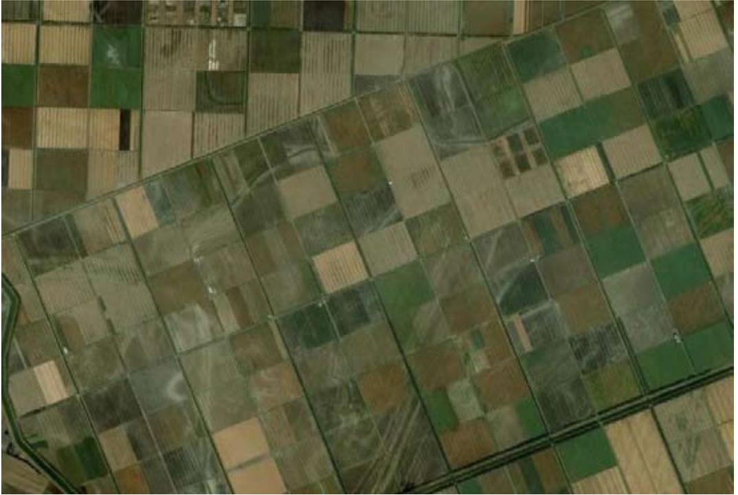
Fig. 2 – Modular division of lands in the “Valle del Mezzano” (Ferrara Province), reclaimed between the ‘50s and the ‘60s of the 20<sup>th</sup> century. Underneath the fields, paleochannels are recognizable. Satellite image. *Source:* Google Earth.
