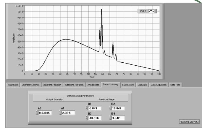
Simulation program of bremsstrahlung and fluorescence lines for tungsten anode. Beam at 100 kVp. The spectrum area must meet the photon fluence measured on-field and be consistent with the instantaneous values measured of the anode current. The model is a modified Birch-Marshall and parameters Bi control the shape of the spectrum, the Ai parameters control the total fluence (area).
