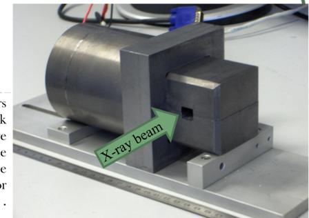
Different Compton spectrometers with different kind of detectors (thick Si, YAP and LaBr<sub>3</sub> scintillator) have been developed and tested. On the right you can see the last prototype made to accommodate a detector based on LaBr<sub>3</sub> scintillator.
