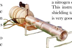
On the left the Compton spectrometer built around a nitrogen cooled HPGe is shown. This instrument is not useful because its alignment and shielding takes very long time but the X-ray spectrometry is very good.
