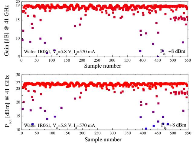
Fig. 5: On-wafer gain and output power mapping of wafer n°1 (554 cells) at 41 GHz,  $P_{in}=+8$  dBm,  $V_d=5.8$  V, and  $I_d=570$  mA.
