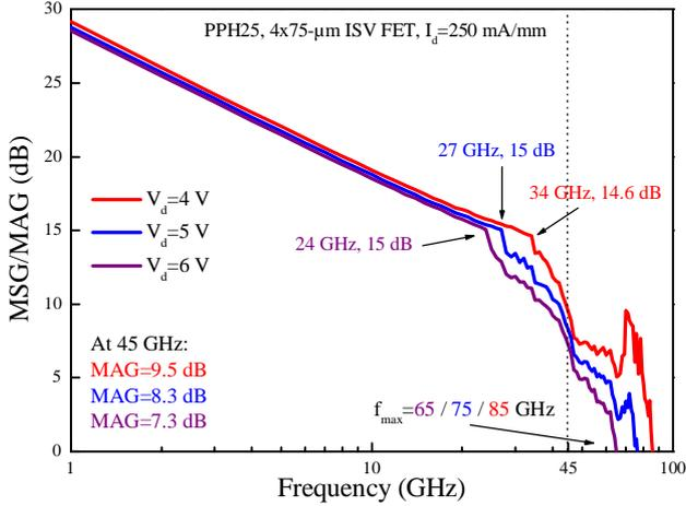
Fig. 1: Measured MSG/MAG of a  $4 \times 75 \mu\text{m}$  ISV PHEMT device at peak transconductance, and  $I_d=250 \text{ mA/mm}$ .
