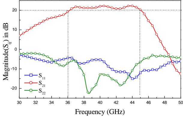
Fig. 4: On-wafer measured small signal gain, input- and output return losses versus frequency of the 35-45 GHz power amplifier at  $V_d=2.0$  V,  $I_d=0.4$  A.
