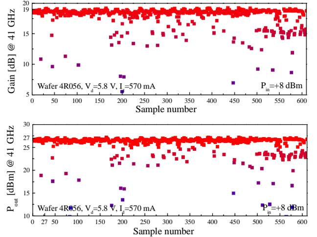
Fig. 6: On-wafer gain and output power mapping of wafer n°2 (608 cells) at 41 GHz,  $P_{in}=+8$  dBm,  $V_d=5.8$  V, and  $I_d=570$  mA.
