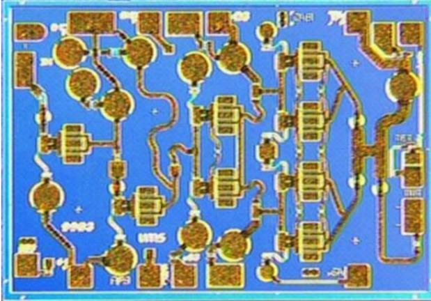
Fig. 2: Chip photograph of the 0.5-Watt 36-45 GHz Power Amplifier MMIC (chip size is  $1.8 \times 1.25 \text{ mm}^2 = 2.25 \text{ mm}^2$ ).
