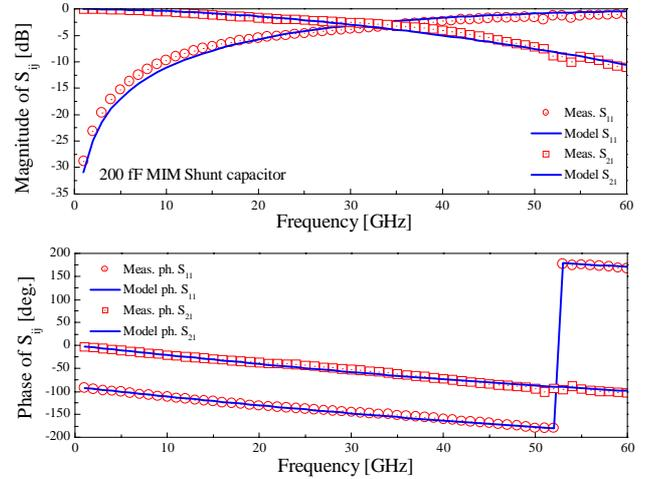
Fig. 3: Comparison between measured and modelled S-parameters of a 200-fF MIM shunt capacitor, over the 0.5-60 GHz frequency range.
