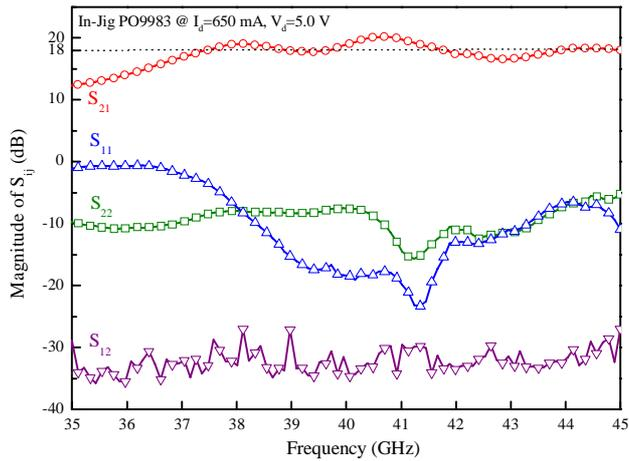
Fig. 7: Measured S-parameters of the JIG test fixtured PA at  $V_d=5$  V, and  $I_d=650$  mA, over the 35-45 GHz frequency range.
