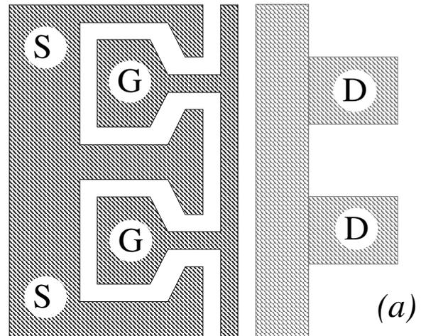
Fig. 2: Schematic topology of Lp7512 (a) and its model (with actual aspect ratio) (b). Part of the source metal is not modeled as unnecessary.
