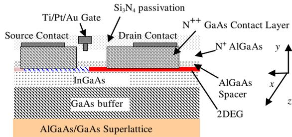
Fig. 1: pHEMT schematic cross-section.
