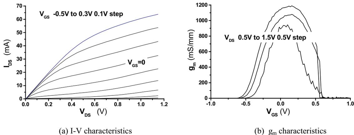
Figure 2 Extrinsic DC output characteristics of 2x50  $\mu\text{m}$  50 nm GaAs MMHEMT
