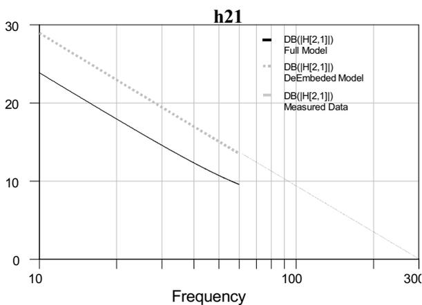
Figure 3 Measured and modeled  $|h_{21}|$  against frequency
