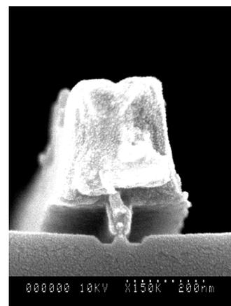
Figure 1 SEM image of the cross section of a fabricated T-gate from a real device.
