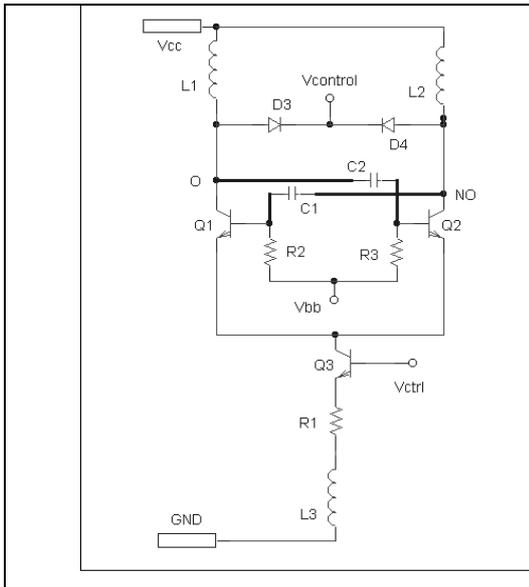
Fig.2- Simplified VCO electrical scheme
