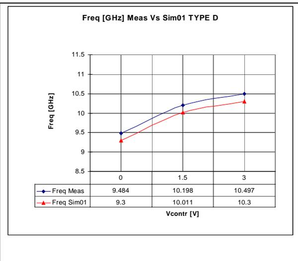
Fig.7- Simulated and measured tuning range
