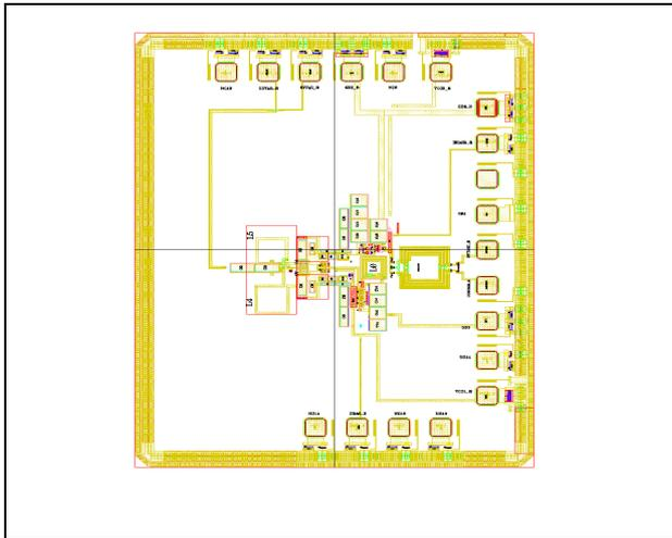
Fig.4- Layout of the SiGe X-Band VCO
