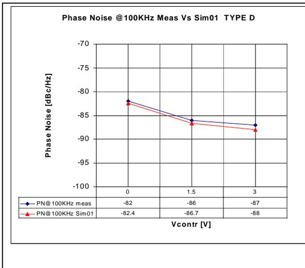
Fig.6- Simulated and measured phase noise
