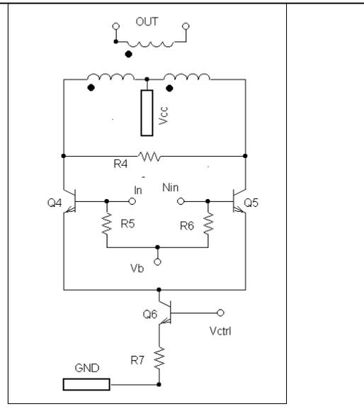
Fig.3- Simplified Buff. and Transformer scheme
