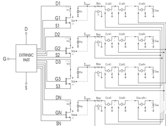
Fig. 2. Simplified schematic of the model for a 2 gate fingers device, showing the extrinsic part, the electrical model and the thermal model
