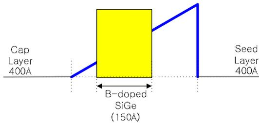
Fig. 2. The standard base profile used.
