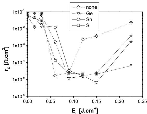
Fig. 1 The dependence of contact resistivity  $r_c$  on energy density of laser radiation  $E_L$  for different doping elements
