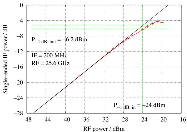
Fig. 7. Input and output -1 dB compression point of the conversion gain at RF = 25.6 GHz and IF = 200 MHz
