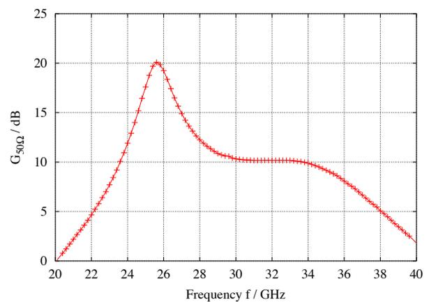
Fig. 4. Gain of the preamplifier in a  $50 \Omega$  test environment
