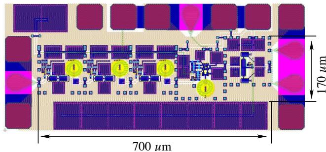
Fig. 2. Layout of the downconverter at 26 GHz ( $700 \times 170 \mu\text{m}^2$ )
