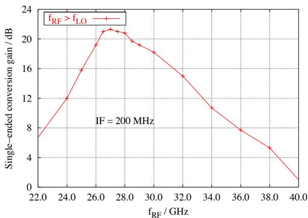
Fig. 6. Single-ended conversion gain of the receiver at a constant IF of 200 MHz
