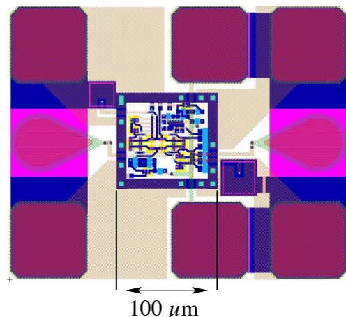
Fig. 9. Layout of the static 2:1 divider (100 × 100 μm<sup>2</sup>)
