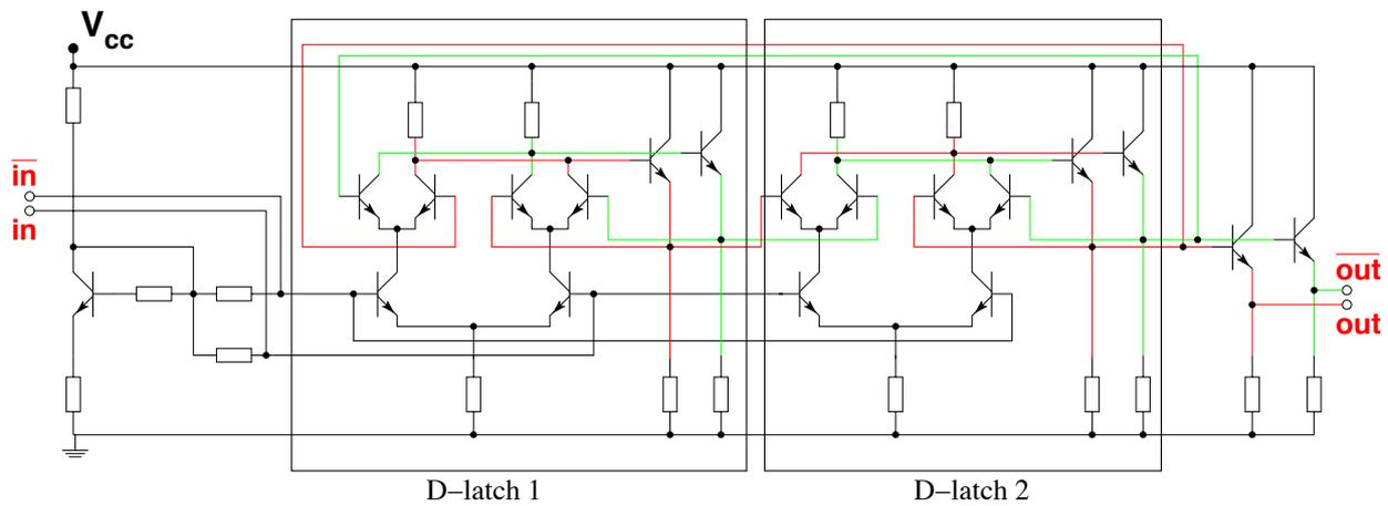
Fig. 8. Circuit schematic of the static 2:1 divider
