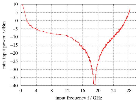
Fig. 10. Input sensitivity for the static 2:1 divider
