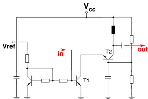
Fig. 3. Circuit schematic of one single stage of the preamplifier
