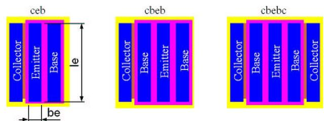
Fig. 1. Electrode configuration of the investigated transistor structures,  $b_e \times l_e = 0.5 \times 19.7 \mu\text{m}^2$  (effective)
