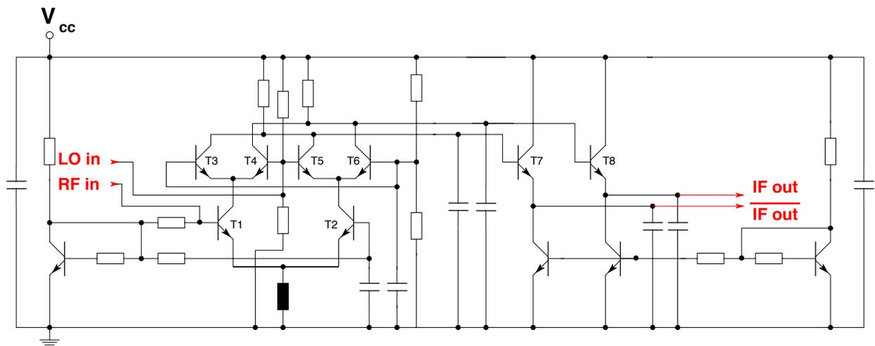
Fig. 5. Circuit schematic of the mixer circuit part
