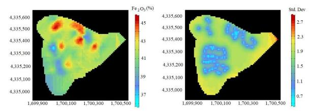
**Figure 8.** Map of Iron variability (wt%) within the Greece bauxite residues (Left) and the estimation precision (standard deviation) map (Right)
