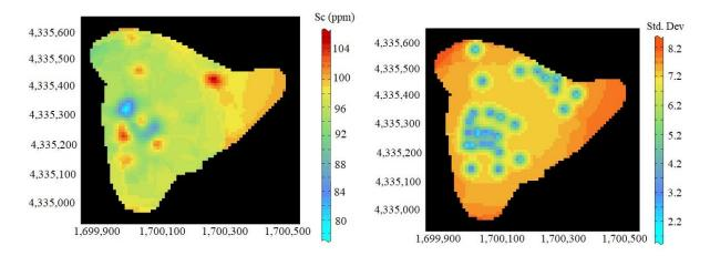
**Figure 11.** Map of Scandium variability (ppm) within the Greece bauxite residues (Left) and the estimation precision (standard deviation) map (Right)
