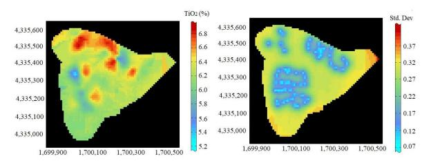
**Figure 10.** Map of Titanium variability (wt%) within the Greece bauxite residues (Left) and the estimation precision (standard deviation) map (Right)
