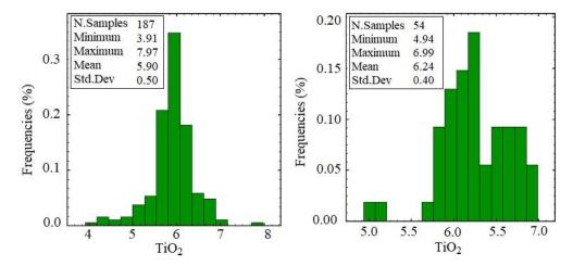
Figure 6. Histograms of data referring to Titanium: daily dumping data from MYT (Left) and the XRF analysis from TU DELFT (Right)
