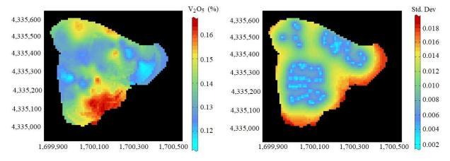
**Figure 9.** Map of Vanadium variability (wt%) within the Greece bauxite residues (Left) and the estimation precision (standard deviation) map (Right)
