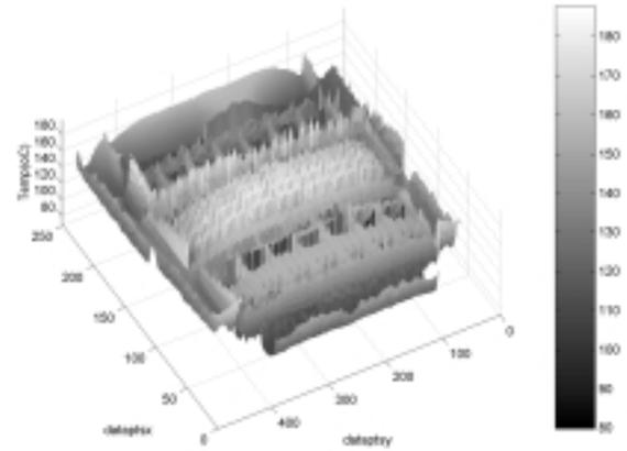
Fig. 5. Emissivity corrected thermal measurement of a power BJT, delivering 250W, in a pulsed class C amplifier configuration.
