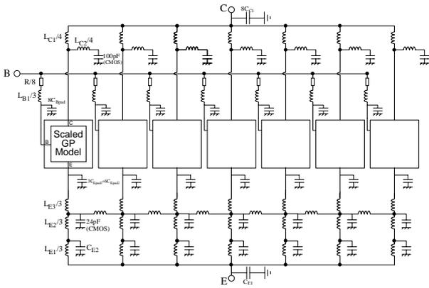
Fig. 2. Example of deconstruction using each die, of a seven die 250W device, as an elementary heat source.
