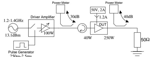
Fig. 4. Measurement set-up used to investigate thermal characteristics associated with pulsed amplifier operation.
