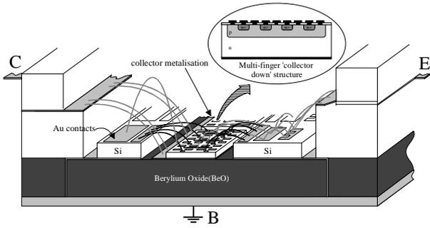
Fig. 1. Complex physical structure of power BJT device.
