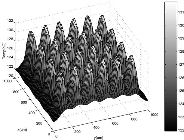
Fig. 3. Simulated thermal distribution across a single isolated die, housing a 6x4 array of transistor devices.
