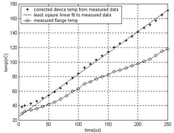
Fig. 6. Measured device temperature variation with pulse width for a fixed pulsing period of 2.5ms.
