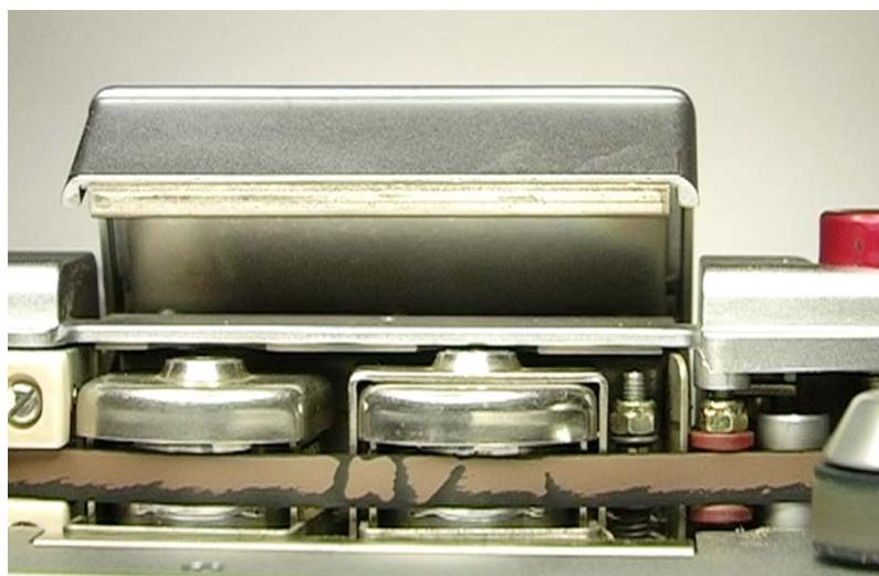
**Fig. 3.** Tape from Luciano Berio's collection during playback on a tape recorder STUDER A810, exhibiting severe magnetic coating shedding.
