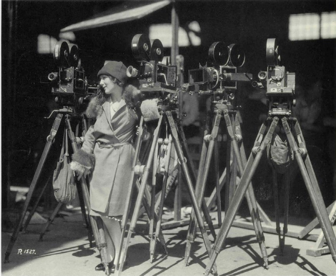
With a coat covering her My Best Girl costume, Pickford stands with a battery of Mitchell cameras. She bought the first Mitchell for her cameraman, Charles Rosher. Third from left is a Bell and Howell 2709.
