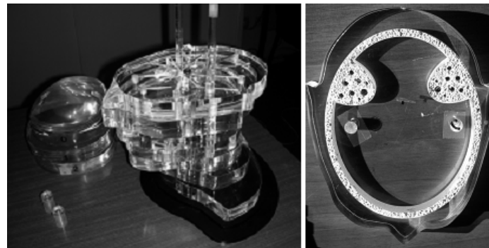
Fig. 3. Pictures of the plexiglass head phantom and of the modified slice with enclosed a geometric hydroxyapatite insert to simulate the skull and the petromastoid part of the temporal bone.
