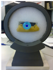
Fig.2. The concentric test tubes sample inside the ESAOTE transmitter/receiver coil.
