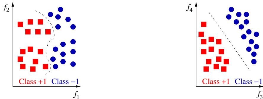
Figure 2.3: Feature extraction. The classification problem is more easily separable using the pair of features f_3 and f_4 (right) than using f_1 and f_2 (left).
