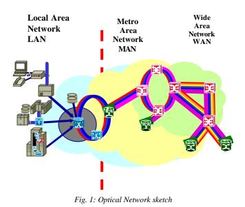
Different network applications mean different requirements for sources and optical components, but some general trends related to: the optimised active material sources (for LAN, MAN and WAN), high speed uncooled sources (mainly for LAN, but also for MAN)
