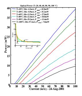
Fig. 2 L-I characteristics of Agilent uncoolad DFB for GbE applications
