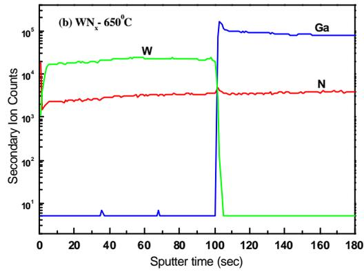
FIG. 4. SIMS depth profiles of the  $WN_x/n$ -GaN contacts after thermal treatments (a) As-deposited. (b) After 650°C RTA annealing. (c) After 850°C RTA annealing.
