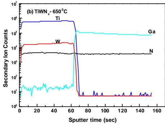
FIG. 3. SIMS depth profiles of the  $TiWN_x/n$ -GaN contacts after thermal treatments (a) As deposited. (b) After  $650^\circ$  RTA annealing. (c) After  $850^\circ$  RTA annealing.
