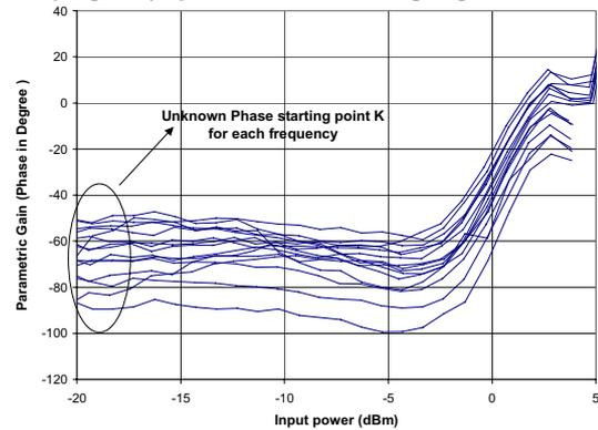
**Fig. 9 :** Phase of Conversion Gain for modulation frequency of +/- 10 MHz around pump carrier
