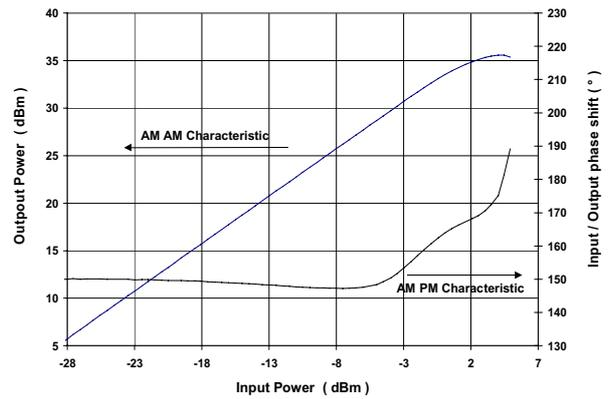
Fig.2 : Power Amplifier AMAM and AMPM Characteristics
