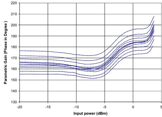
**Fig. 7 :** Phase of Parametric Gain for modulation frequency of +/- 10 MHz around pump carrier
