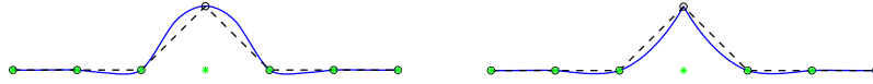
Figure 9: Basis function of the NULI 4-point scheme with uniform knots, edge parameters \lambda_{i-1}^0 = 0.1, \lambda_i^0 = 0.9 (left)/ \lambda_{i-1}^0 = 1, \lambda_i^0 = 0 (right) and tagged vertex (x_i, 1) .
