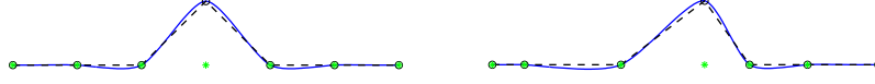
Figure 8: Basis function of the NULI 4-point scheme with uniform knots (left) and non-uniform knots (right). The edge parameters are set to \lambda_i^0 = \frac{1}{2}, \forall i .
