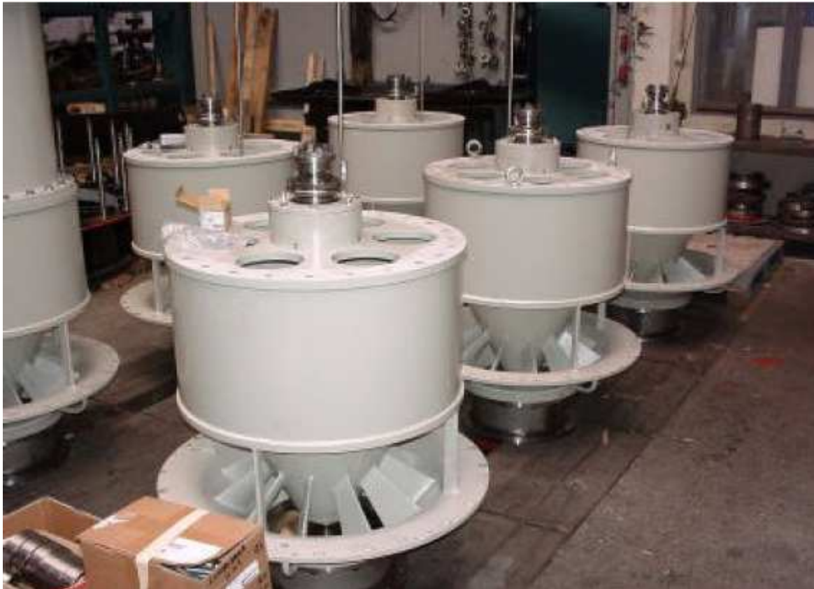
Figure 16: The six axial propeller turbines being assembled at Kössler GmbH
