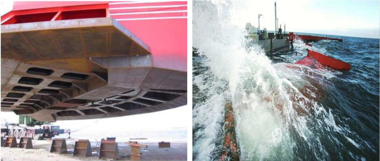
Figure 15: On the left WD prototype at launch in March 2003: the open air-chambers are used to control the floating level. On the right WD prototype in heavy wave conditions.
