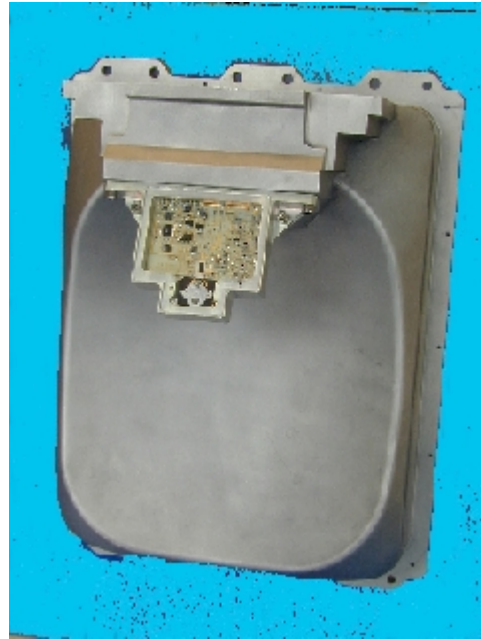
Fig 2: Front view of the complete transceiver, radome removed, front-end cover removed. The overall dimensions are approximately: 22 x 30 x 15 cm
