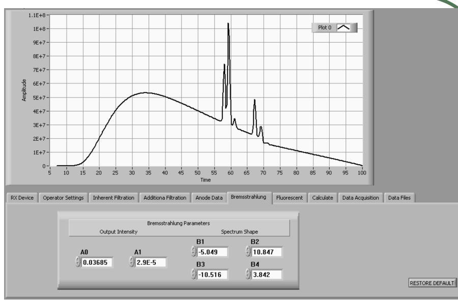
Simulation program of bremmstralhung and fluorescence lines for tungsten anode. Beam at 100 kvp. The spectrum area must meet the photon fluence measured onfield and be consistent with the instantaneous values measured of the anode current. The model is a modified Birch-Marshall and parameters Bi control the shape of the spectrum, the Ai parameters control the total fluence (area).
