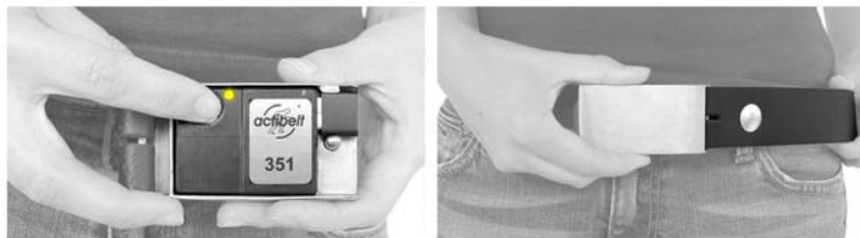
Figure 1. Photos of the actibelt® accelerometer used for the data acquisition.
