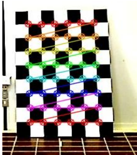
Figure 3. Flat planar pattern used in the calibration procedure; internal corners are detected automatically and colour-marked to show the positive matches resolved by the software.
