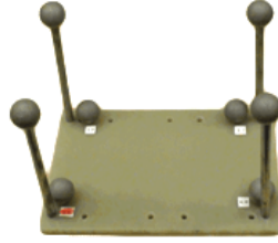
Figure 1: Fixture used to calibrate the MaxTRAK system. (Approximately 200 x 100 x 150 mm)
