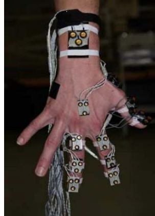
Figure 1. Marker set used to record kinematic data of the forearm and the thumb, index and middle fingers.
