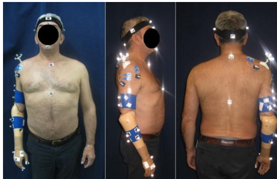
Figure 1 Marker-set for the motion analysis based on an optoelectronic system
