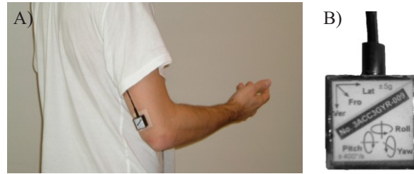
Figure 1. Measurement system: A) Inertial modules attached to the dorsal part of humerus and to the sternum; B) Detail of an inertial module with tri-axial gyroscope and accelerometer.
