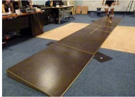
Figure 2: Cross-slope device instrumented with four force platforms
