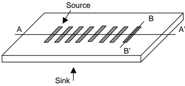
Fig. 2. 3D structure of 8 finger HBT.
