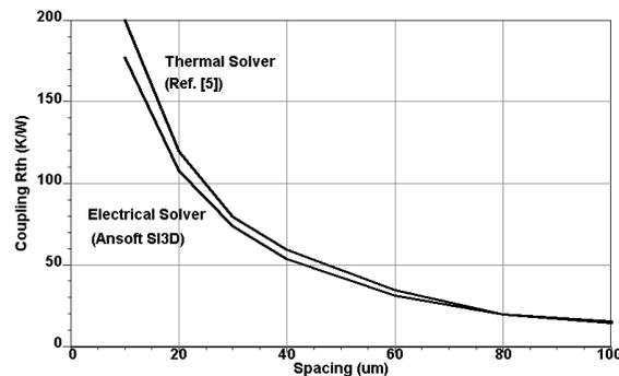
Fig. 1. Extracted coupling thermal resistance using thermal and electrical field solvers
