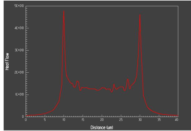
Fig. 5 Heat flow distribution along BB' in Fig. 2
