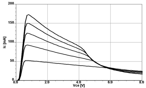
Fig. 7. Calculated collector current in a 5-finger HBT under constant base current, the base current levels are 0.5, 1.0, 1.5, 2.0 and 2.5mA.
