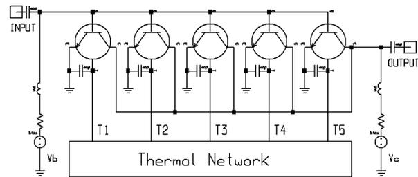
Fig. 6 Electro-thermal model of multi-finger HBT, the nodes voltage T1...T5 equals the temperature rise inside each HBT
