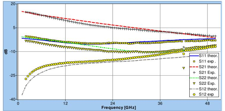
Fig. 3: Comparison between calculated and measured data for pHEMT LP7512.
