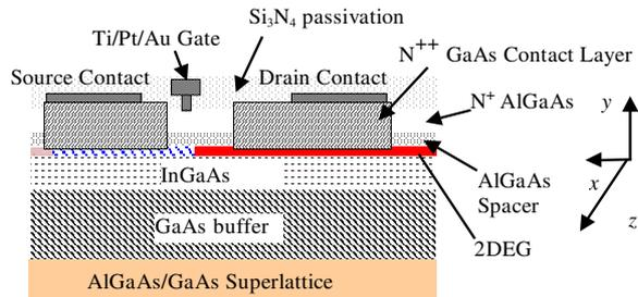
Fig. 1: pHEMT schematic cross-section.
