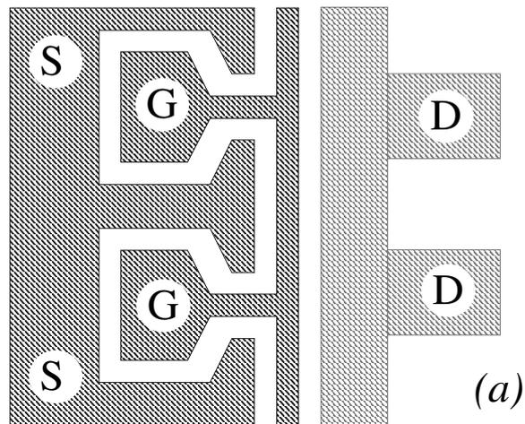
Fig. 2: Schematic topology of Lp7512 (a) and its model (with actual aspect ratio) (b). Part of the source metal is not modeled as unnecessary.
