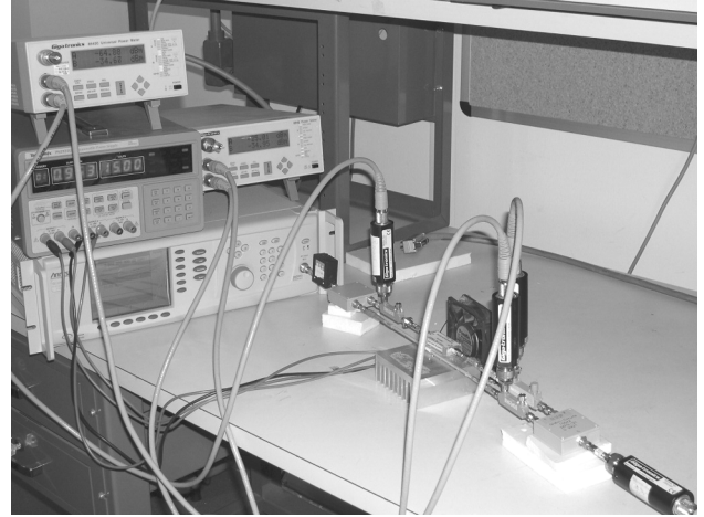
Fig. 3 : Photo of the measurement set-up for the Am-Am and Am-Pm characterization.
