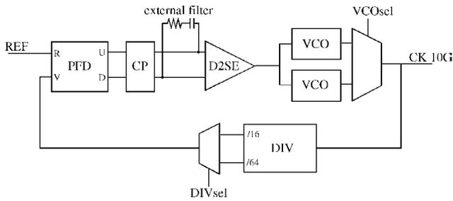
Fig. 1. CMU IC functional block diagram.
