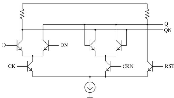
Fig. 4. D-latch with reset for the PFD.
