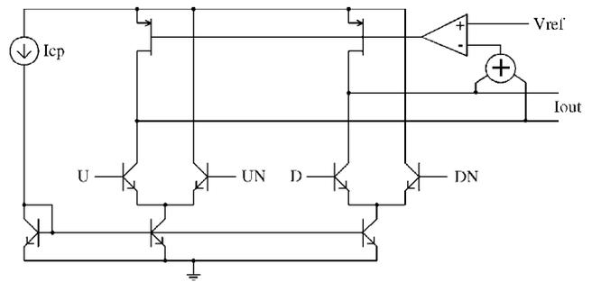
Fig. 5. Differential charge pump.
