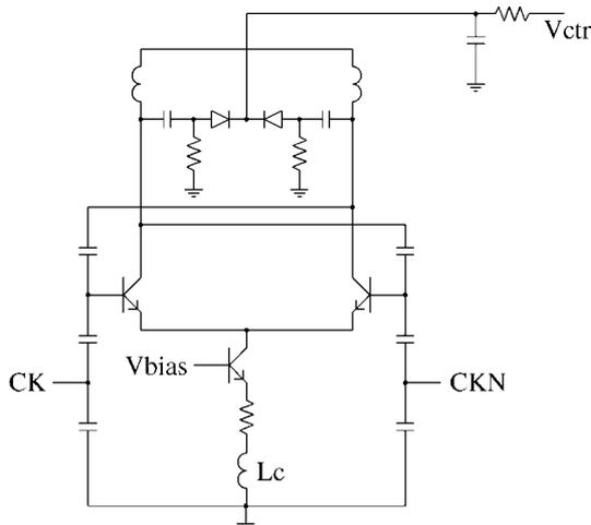
Fig. 2. Voltage-controlled oscillator.
