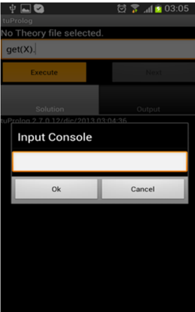
Figure 3.30: Keyboard input management in the case of a read operation from the standard input.
