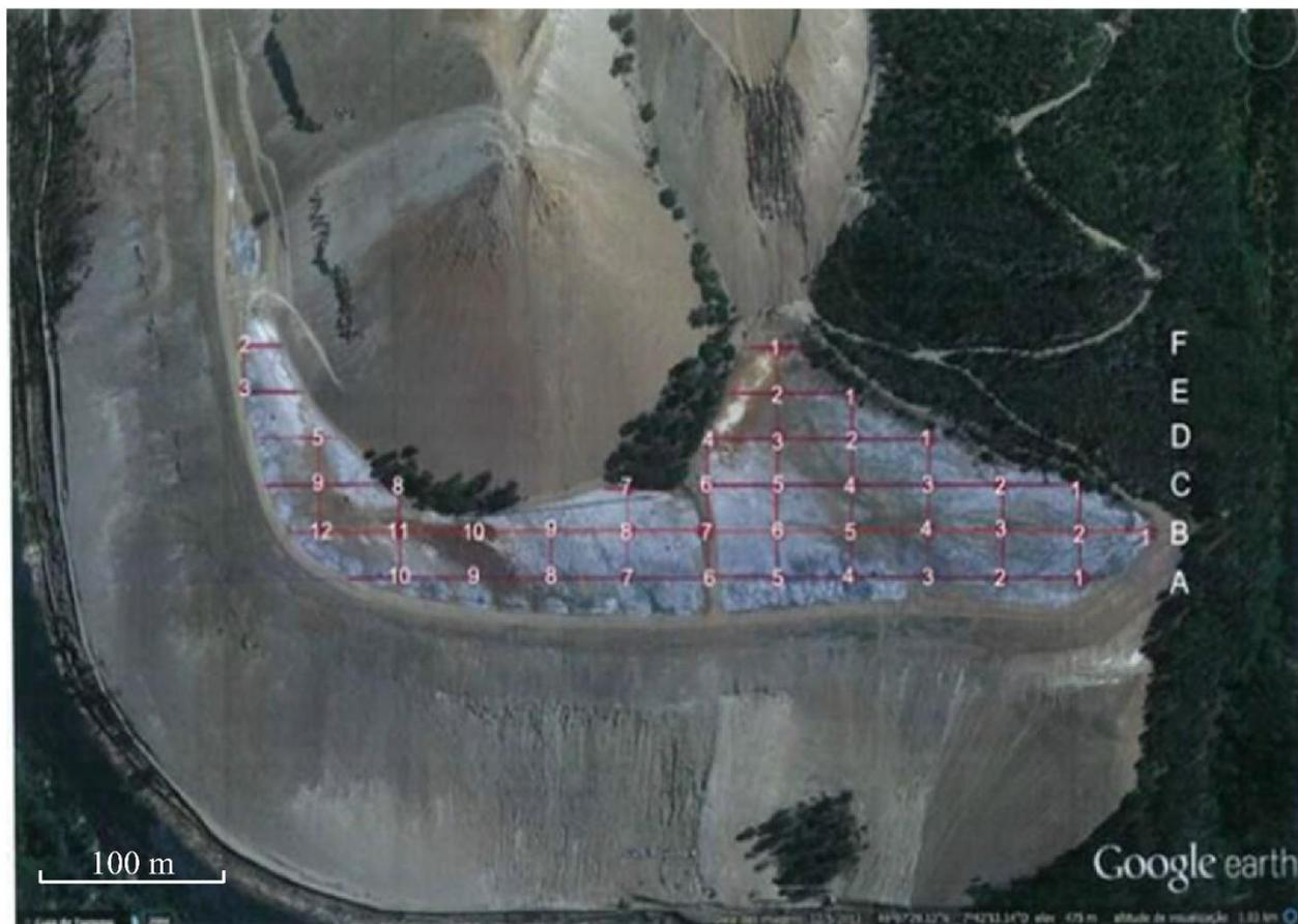
**Figure 2.1. Localization of the soil samples grid – 41 red dots, disposed over 6 lines – inside the tailings dam of the Cabeço do Pião mine for the period November 2016 to December 2017 (from De Lurdes Dini, 2019)**
