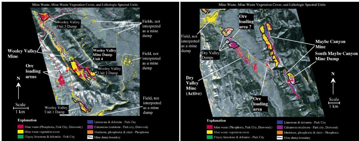
**Figure 4.3. AVIRIS image of the Wooley Valley Mine (left) and the Maybe Canyon Mine (right) with lithologic and mine waste spectral units, and interpreted mine dumps mapped in black lines (from Mars and Cowley, 2003).**
