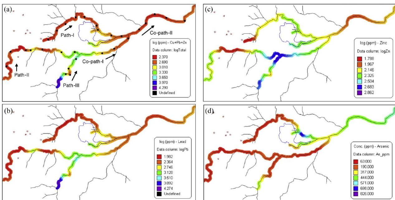
**Figure 4.1. Streamlines and maps of concentration of heavy metals (Pb, Zn and As) obtained by comparison between samples and hyperspectral images for the Rodalquilar mining area, Spain.**
