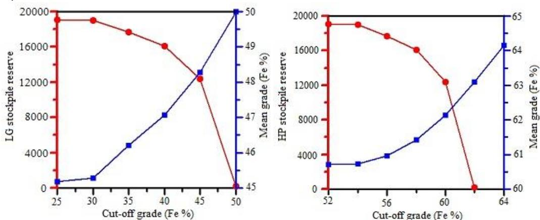
**Figure 3.3. Grade-Tonnage curve for two simulated stockpiles (from Kasmae et al., 2018)**
