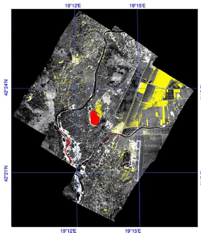
**Figure 4.2. Red Dust (RD) map as attained by applying ISODATA clustering to the chosen IC bands; yellow and red colours show the RD on soils and the RD on water classes, respectively (from Pascucci et al, 2012).**
