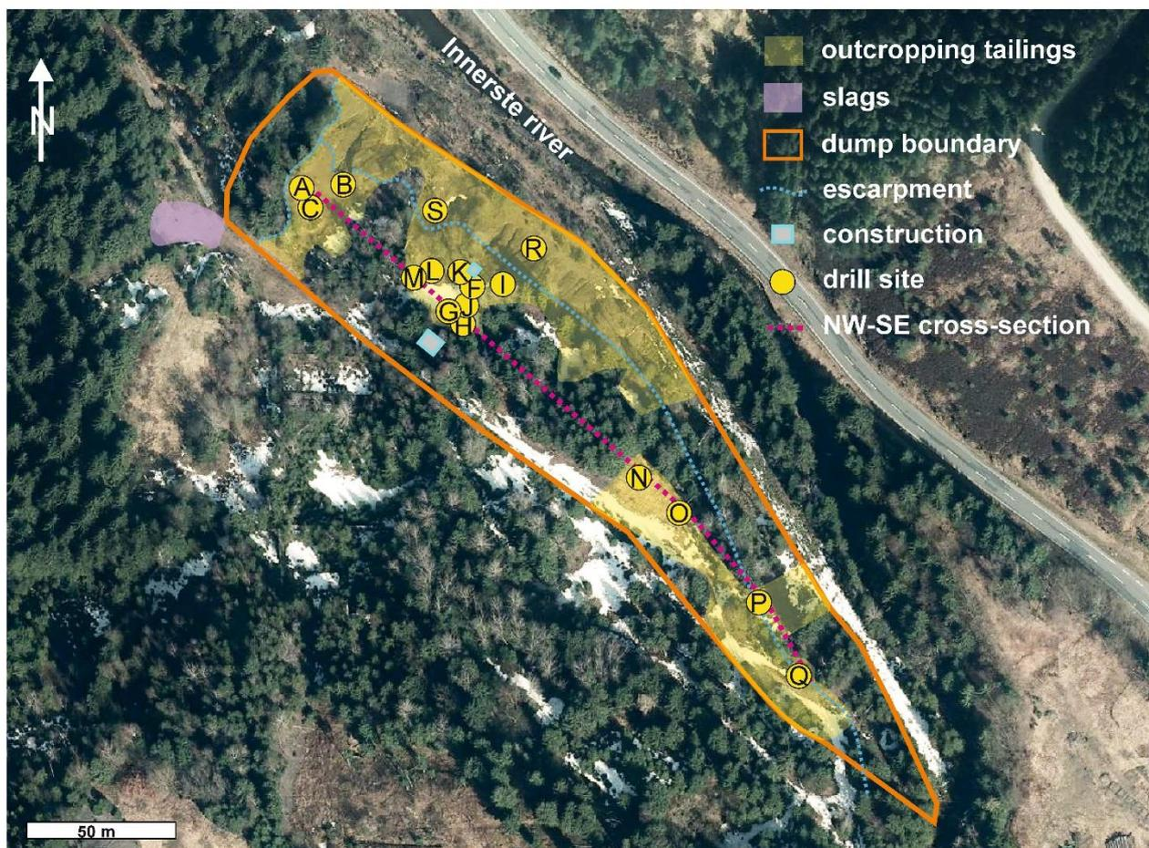
**Figure 2.2 Localization of the drilling samples (yellow dots) over the historical and revegetated mining waste area (from Kuhn and Meima, 2019)**
