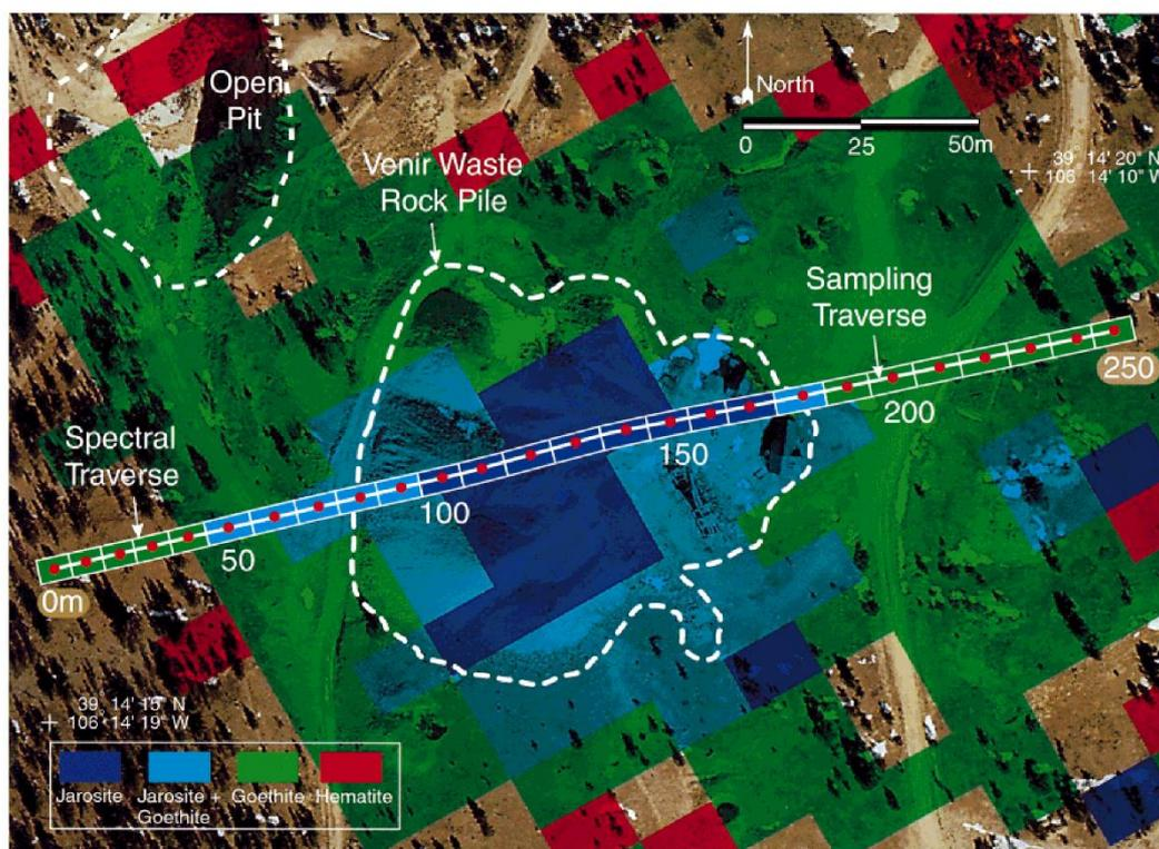
**Figure 4.5. Spectral traverse and AVIRIS mineral maps overlaid on a high-spatial-resolution aerial photograph of the Venir traverse mine waste (from Swayze et al., 2000)**
