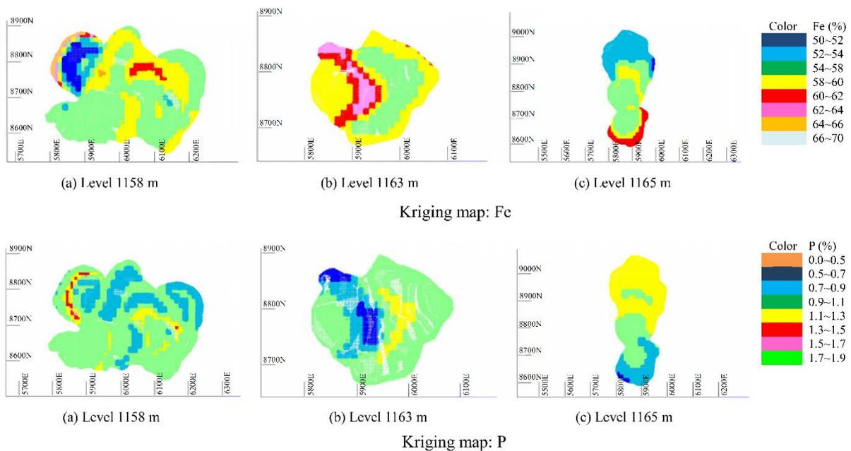
**Figure 3.2. Maps of iron and phosphorous variability in three levels of HP stockpiles (from Kasmae et al., 2010).**
