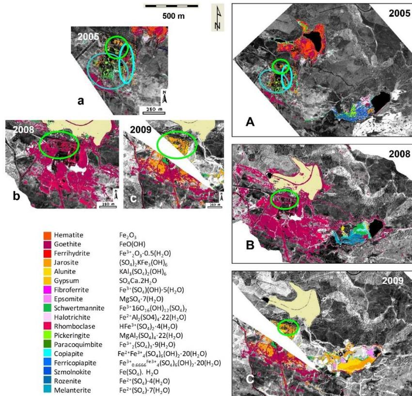
**Figure 4.4. Mineral variations in the period 2005-2009 in the mining site of Sotiel, Spain, obtained by the analysis of hyperspectral data (from Buzzi et al., 2014)**
