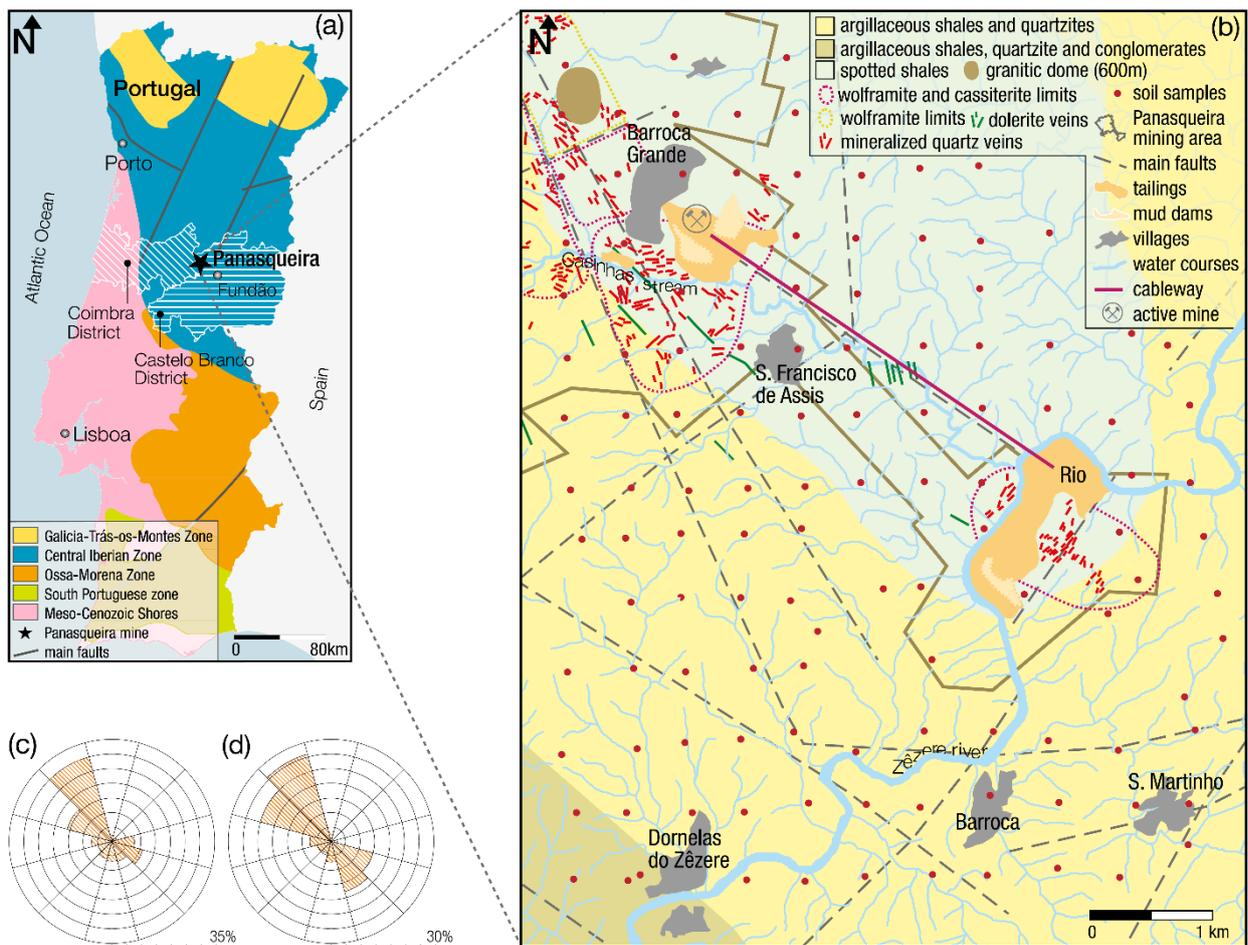
**Figure 1.3** Localization of the soil samples grid - 122 red dots – (b) inside the study area (a), considering the wind rose diagram on the top of the Barroca mine (c), and on the top of the mountain 800 m north to the mine (d). (from Candeias et al. 2014)
