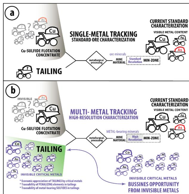
**Figure 5.1. Multi-Metal Tracking approach in comparison to traditional single-metal tracking (from Velásquez, 2020).**
