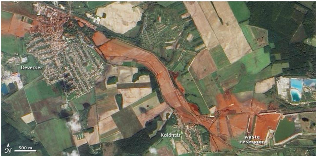
**Figure 2. Broken bauxite tailing dam causing spill and pollution spread in Hungary**
