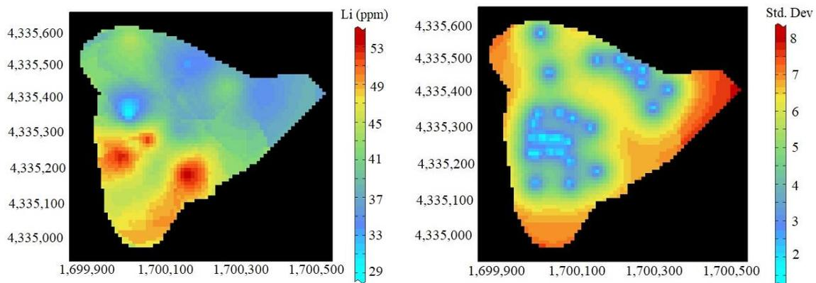
**Figure 12.** Map of lithium variability (ppm) within the Greece bauxite residues (Left) and the estimation precision (standard deviation) map (Right)
