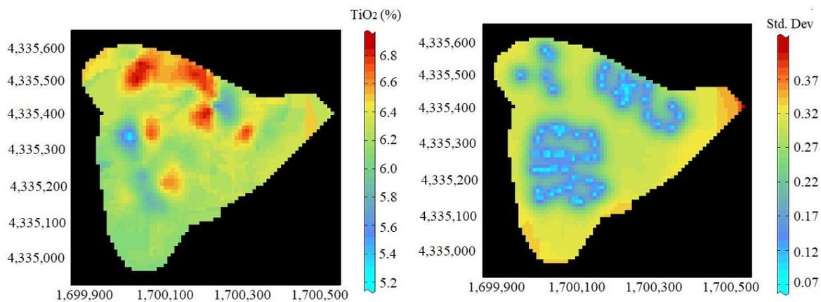
**Figure 10.** Map of Titanium variability (wt%) within the Greece bauxite residues (Left) and the estimation precision (standard deviation) map (Right)
