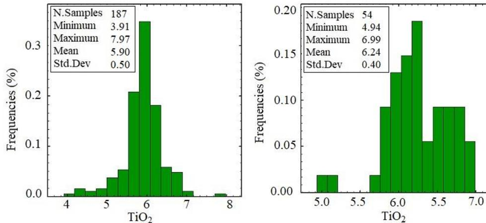
**Figure 6.** Histograms of data referring to Titanium: daily dumping data from MYT (Left) and the XRF analysis from TU DELFT (Right)
