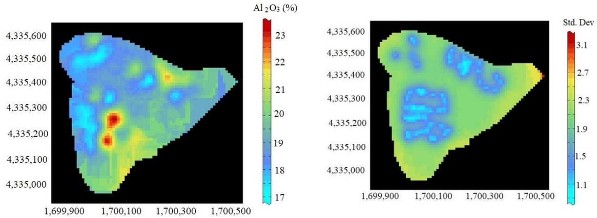
**Figure 7.** Map of Aluminium variability (wt%) within the Greece bauxite residues (Left) and the estimation precision (standard deviation) map (Right)
