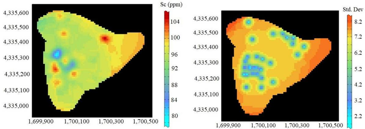
**Figure 11.** Map of Scandium variability (ppm) within the Greece bauxite residues (Left) and the estimation precision (standard deviation) map (Right)
