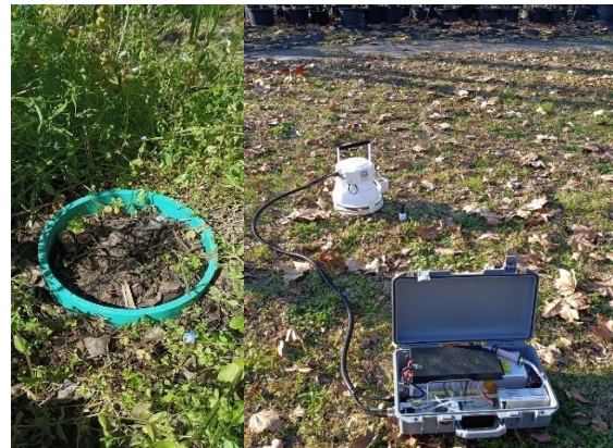
Fig. 2 – Measurement apparatus for N 2 O fluxes on the pear orchard field: on the left, chamber collar inserted in the soil, on the right the dynamic chamber attached to the portable measuring system LI-7820.
